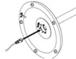
Step 4: Place the power cord plug through base, bottom pole, middle Pole and top pole. Connect the power cord plug to the socket in the heater head.
