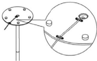
Step 7: Raise or retract the top telescopic tube to the desired height and tighten to the middle tube by screwing knob down.
