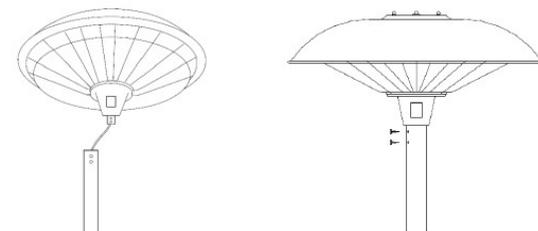
Step 6: Pull the power cord gently out of the base as much as possible. Fix the power cord under the weighted base using the supplied 4pcs M4 nuts.
