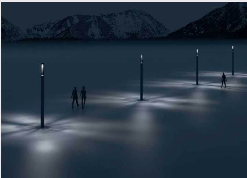
Simulation Screen 751311 38W 3000K Optics 360° Luminares interdistance 12mt.
