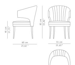
DIMENSIONS WIDTH DEPTH HEIGHT SEAT HEIGHT SEAT DEPTH ARMREST HEIGHT 55 cm | 21,65" 60 cm | 23,62" 85 cm | 33,46" 43 cm | 16,93" 45 cm | 17,71" 70 cm | 27,55"
