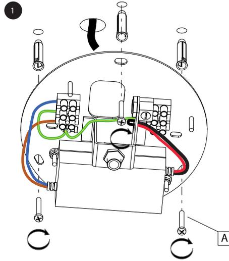
**EN** Drill holes in the ceiling positioned according to the template of the ceiling rose and install the screw anchors. Fix the ceiling rose into the ceiling with screws (A).
