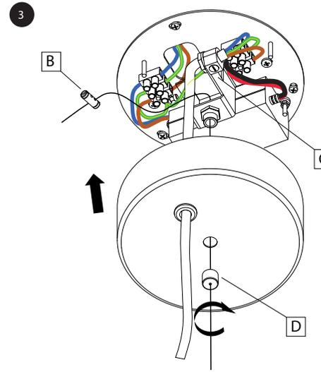
**EN** Hang the lamp module by the steel wire suspension cable as shown in the diagram, and adjust to desired height using clamp (B). Secure the electrical cable to the lamp using clamp (C). Fit the rose cap and secure it with the knurled screw (D).
