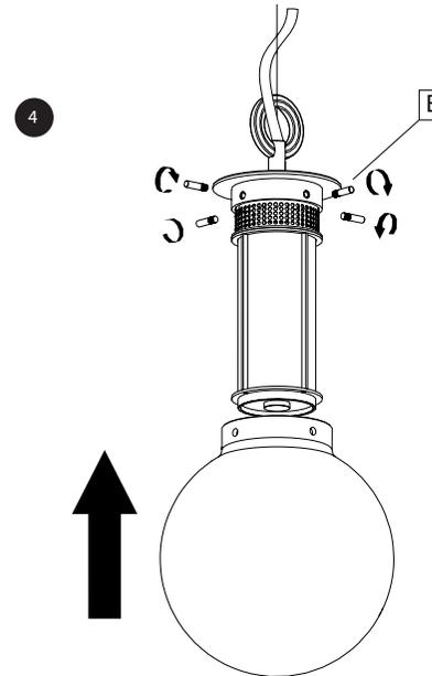
**EN** Unfasten the headless screws (E) from the main body of the lamp module, position the diffuser and then re-fasten the screws (E) to hold it in place.
