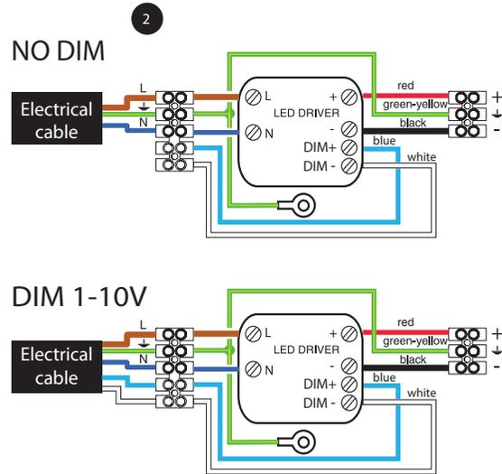
**EN** Connect the lamp to the mains according to the wiring diagram.
