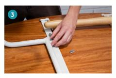
To fix the leg we need 1 screw, 2 washers and 1 nut. Before tightening the screws we must place them on both sides of the legs. The screw head must be placed on the outer side.
