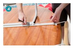
To tighten the screws we will need a wrench  $n^2$  13 and an Allen key  $n^2$  6.
