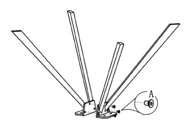
Note: Just pre-tighten screws(A) in Step 1.
