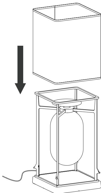
EN Place the diffuser again on the structure and leave it supported.
