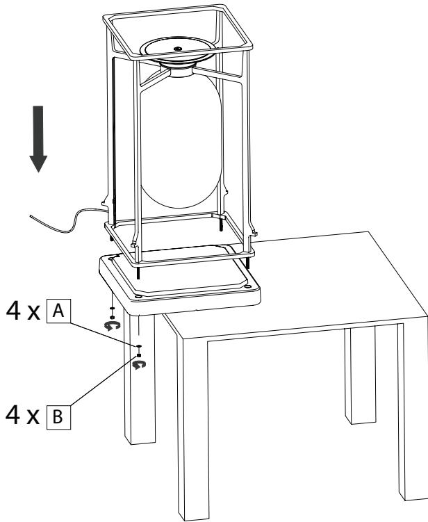
EN To facilitate assembly, support the base of the luminaire on a raised surface previously protected to avoid scratching. Put together the lighting fixture structure with the concrete base and fix it with the washers (A) and the nuts (B).
