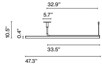
“(1) The height can be increased by means of the 15.7 or 23.6” poles (max. 3 units.) They can be combined.”
