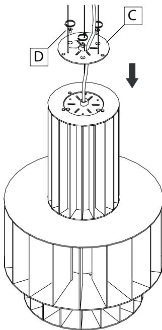
**EN** Attach the top cover (C) and fasten to the electric group with screws (D).
