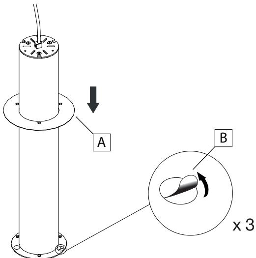
**EN** Slide the disc (A) onto the electric group and line up the three holes with the lugs at the base of the electric group. Fix the disc onto the base by removing the plastic covering the adhesive stickers (B).
