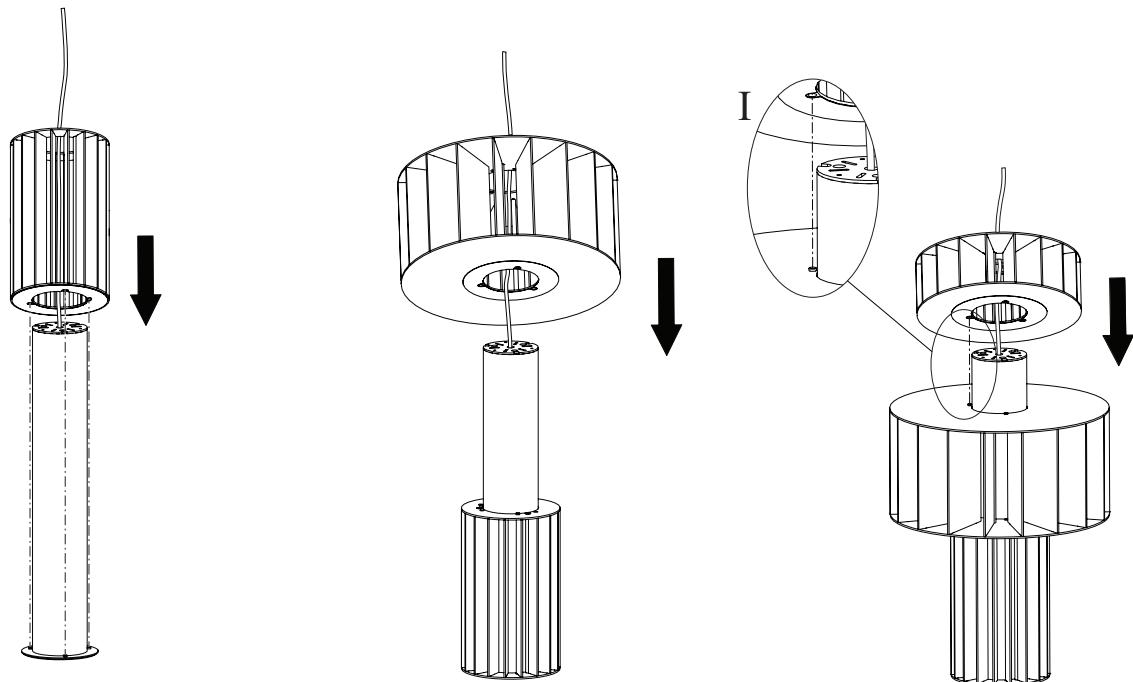
**EN** Slide the first module onto the electric group, as applicable to the model purchased (Bable PE, ME GR o CUSTOM), making sure that the holes line up with the lugs at the base (detail I). Repeat this step according to the order, colour and quantity needed to complete the lighting.
