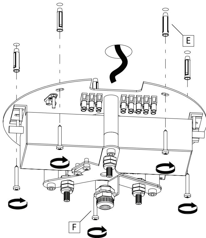
**EN** Drill holes in the ceiling positioned according to the template of the ceiling rose and install the screw anchors (E). Fix the ceiling rose into the ceiling with screws (F).
