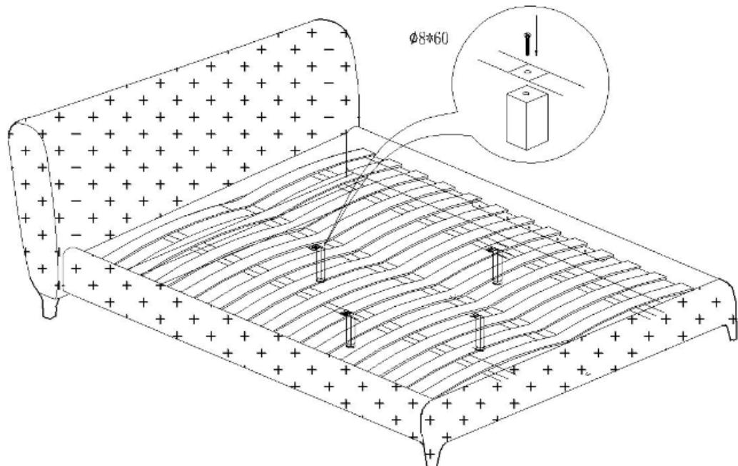
3: lock the slat feet by 8\*60 flat head screws.put the bed slat on the triangle supporter .
