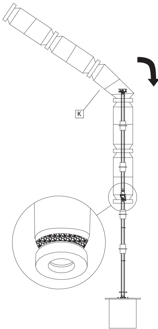
**EN** Place shade (K) carefully on to the light structure. Note that there is a specific way to place the shade. Ensure that the end with the black tape goes over first. Once the correct end has been identified, remove the tape. When placing the shade, it is necessary to stretch the fabric to fit over the components (N), do it without fear.
