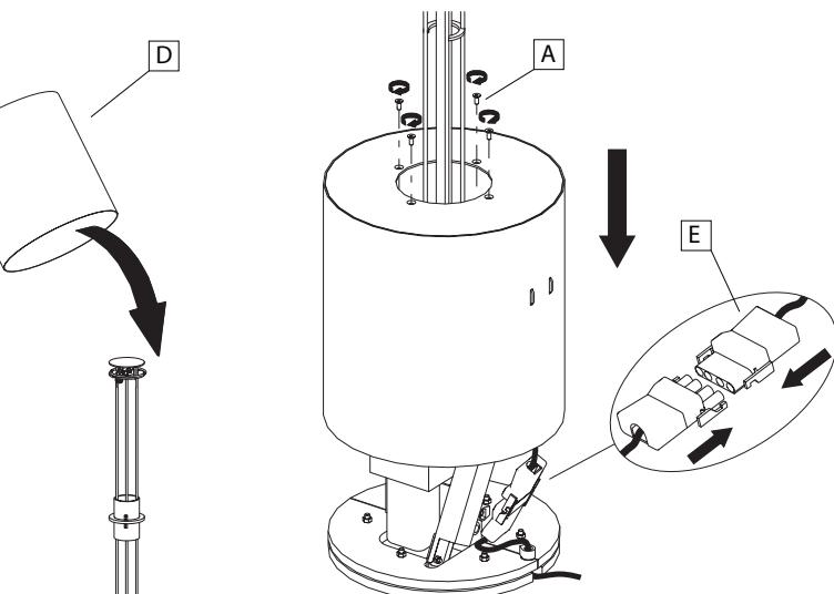
**EN** 7.1 Position the cylinder that covers the body of the base (D), connect the connectors (E) and fix with screws (A).
