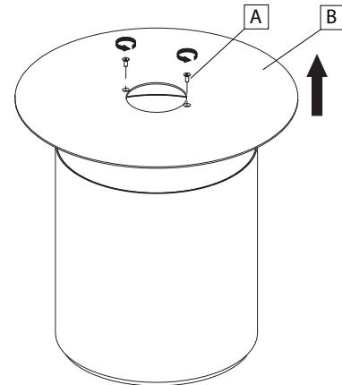
**EN** Unscrew the screws (A) and remove disc (B).
