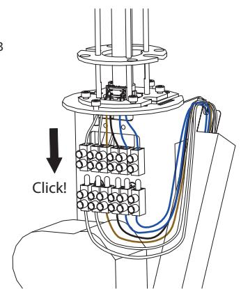
**EN** 3.1 Position the structure (I) with the interval body of the base, passing the connectors through it, in "FRONT" position.
