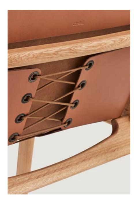
The seat and backrest are made of a leather cover with the extreme parts of the cover sewn, with painted edges for a high-quality and perfect finish. The other halves of the sheath are closed like a corset, with eyelets and a 4mm diameter nylon cord. The part of the eyelets is internally reinforced with stainless steel plates, to keep the bag flat and not deform with the tension of the stringing.
