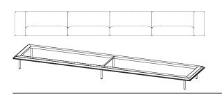
Structural sofa frame made of extruded aluminum profile with 6 legs made of steel rod. The legs can be assembled in different positions.
