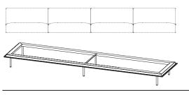
Structural sofa frame made of extruded aluminum profile with 6 legs made of steel rod. The legs can be assembled in different positions.
