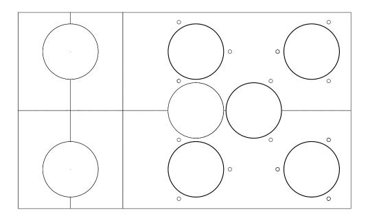
2 Once all the legs are placed, rotate them until they align with the small holes in the templates.
