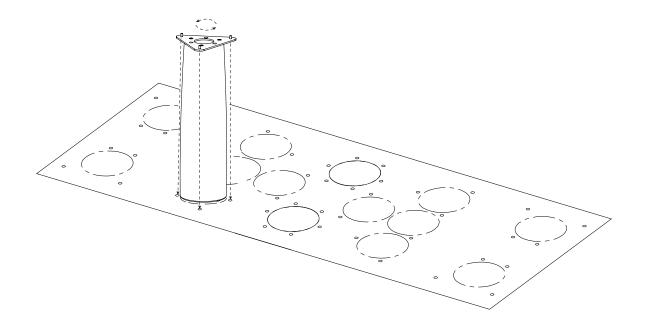
4 Unscrew the center leg plates and screw on the dual mounting kit.
