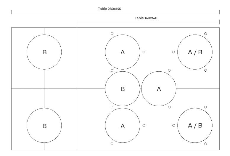
( 1 ) Place the template sheet on the ground and place the legs in the bold positions
